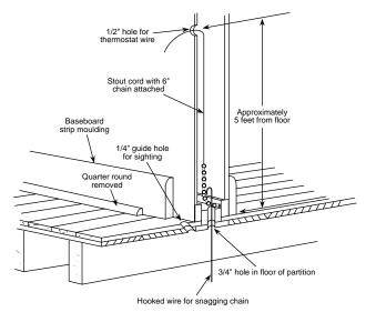
Figure 1. Routing thermostat wires
